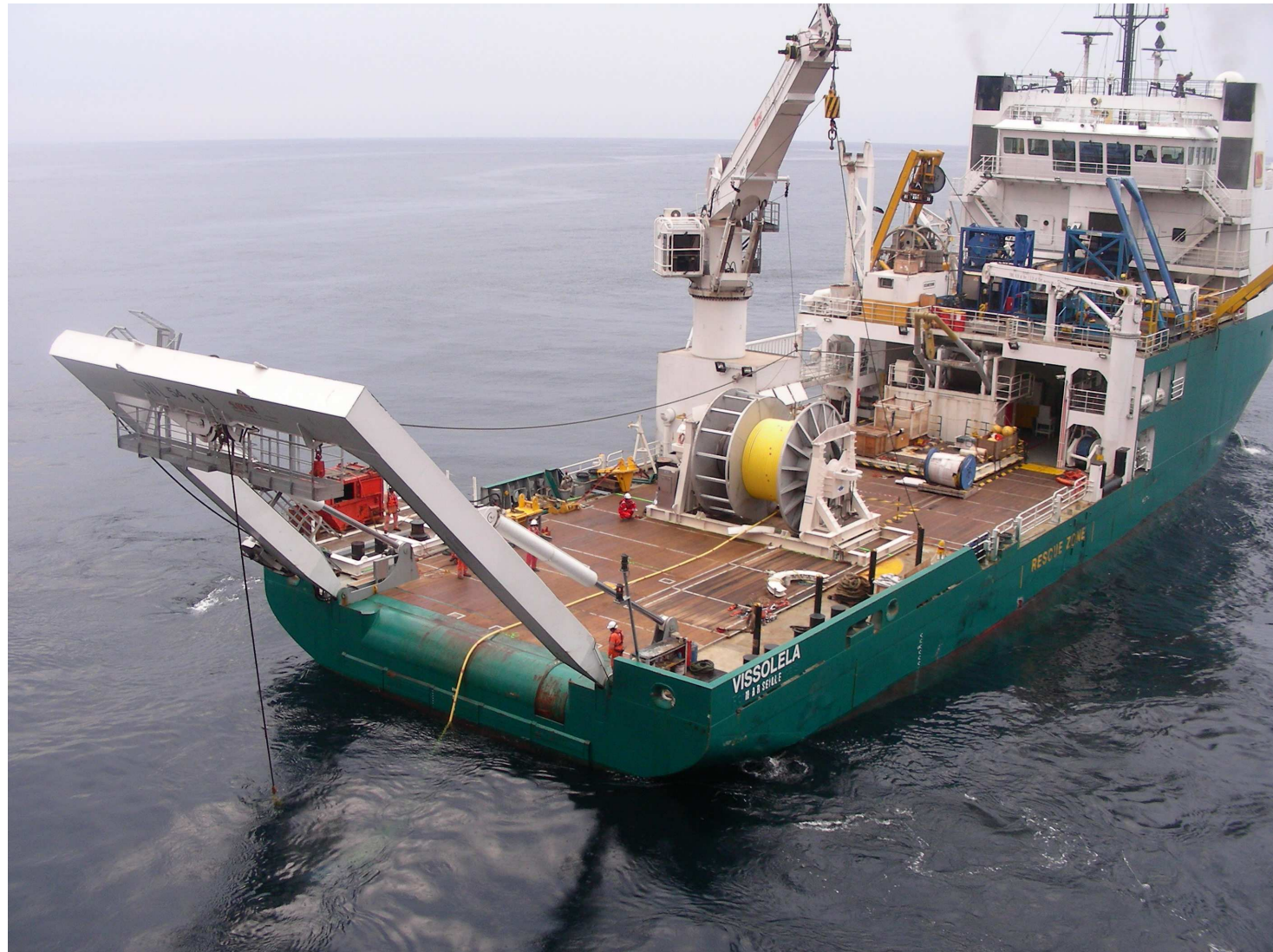
Source : BOURBON - "Vissolela", umbilical deployment - 1400 meters water depth in Equatorial Guinea - Client Exxon
